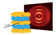
Spontaneous formation of smectic and columnar structures was observed when spherical gold nanoparticles were functionalized with mesogenic thiols (see layered structure and X-ray pattern of a sample in smectic phase). The particle ordering is stimulated by softening of the interparticle potential and flexibility for deformation of the grafting layer.
