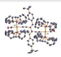
Tungsten tryst: A 4-H-butatrienylidene complex of tungsten was successfully isolated and structurally characterized. It undergoes a unique self-coupling, which leads to a dimer (see picture; P pink, O red) with a cross-conjugated  $\pi$  system and with electrochemically and magnetically active metal centers.
