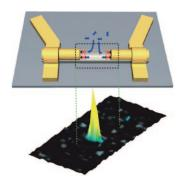
Click to fill the gap: The in situ modular fabrication of molecular transport junctions in nanogaps generated by on-wire lithography is achieved by using click chemistry (see picture). The formation of molecular junctions proceeds in high yields and can be used to test different molecules; the triazole group also maintains conjugation in the molecular wires. Raman spectroscopy is used to characterize the molecular assembly processes.
